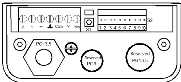
**Manual self-adaption:** Press and hold button S1 on PCB for more than 5s (See Fig. 1) until the indicator starts blinking (1Hz) to enter into self-adaption mode. The phenomenon will be the same as power-on self-adaption.
